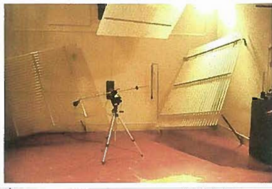
Figure 12 Barrier absorption: Reverberation Room Method photo #2553
